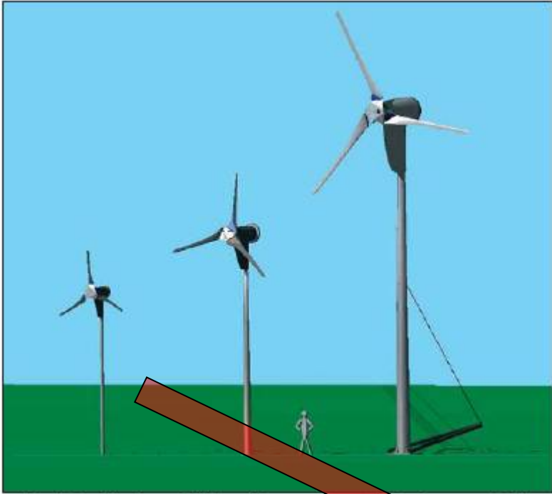
From left to right Proven 2.5kW on 6.5m tower; Proven 6kW on 9m tower; 6ft tall man and Proven 15kW on 15m tower
